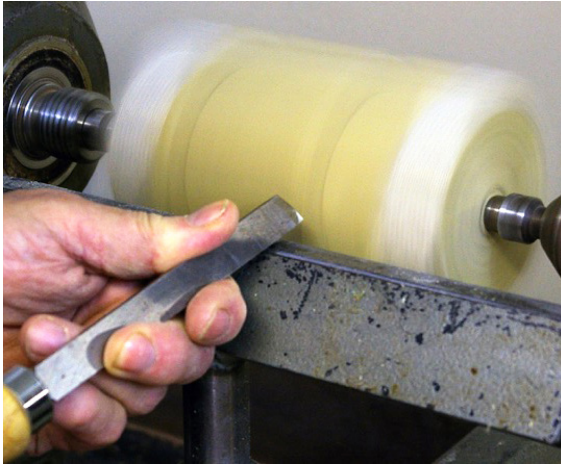
(Fig. 2) Carefully make V-cuts with the point of a skew to establish the ends of the cove.
